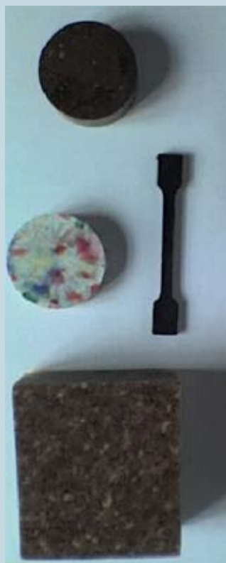
Figure 2. Rack-wheels from recycled capron (above); phenolformaldehyde resin and mineral filler (below, left); tube manufactured from recycled polypropylene filled with graphite (below, right)
